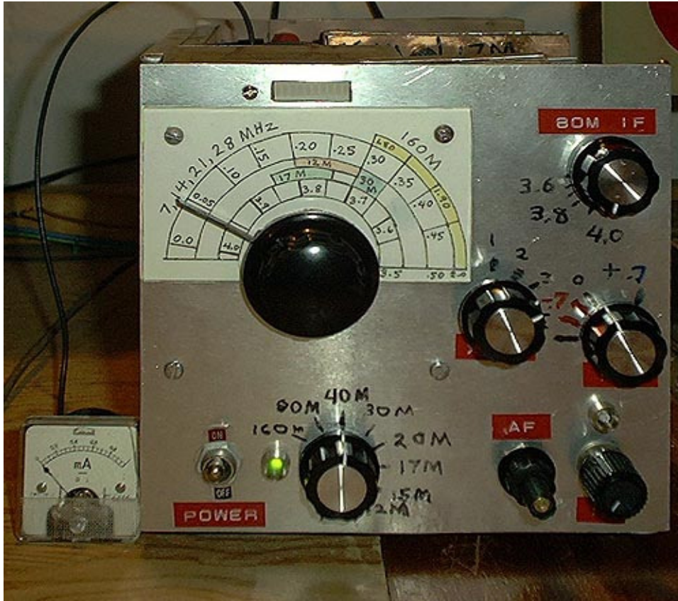
Homebuilt all-band dual conversion HF ham receiver.
