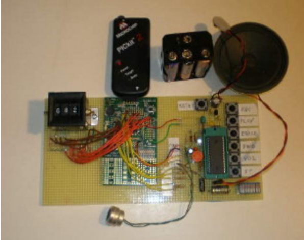
A PIC16F887 development board wired into a speech chip programmer. The black plastic programmer unit is plugged into the development board.
