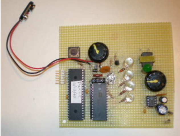
A PIC16F887 breadboard for developing software to drive the speech chip. Note the 6 pin connector on the left used to program the large, 40 pin PIC microcontroller.
