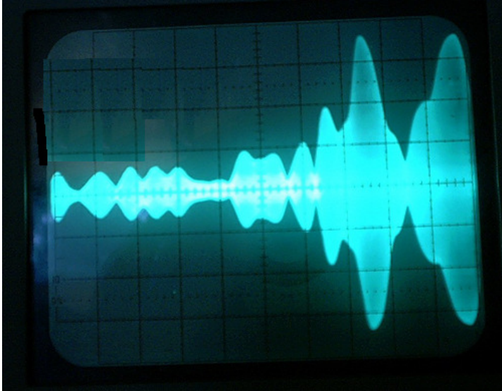
The 9 MHz SSB voice signal seen on an oscilloscope.
